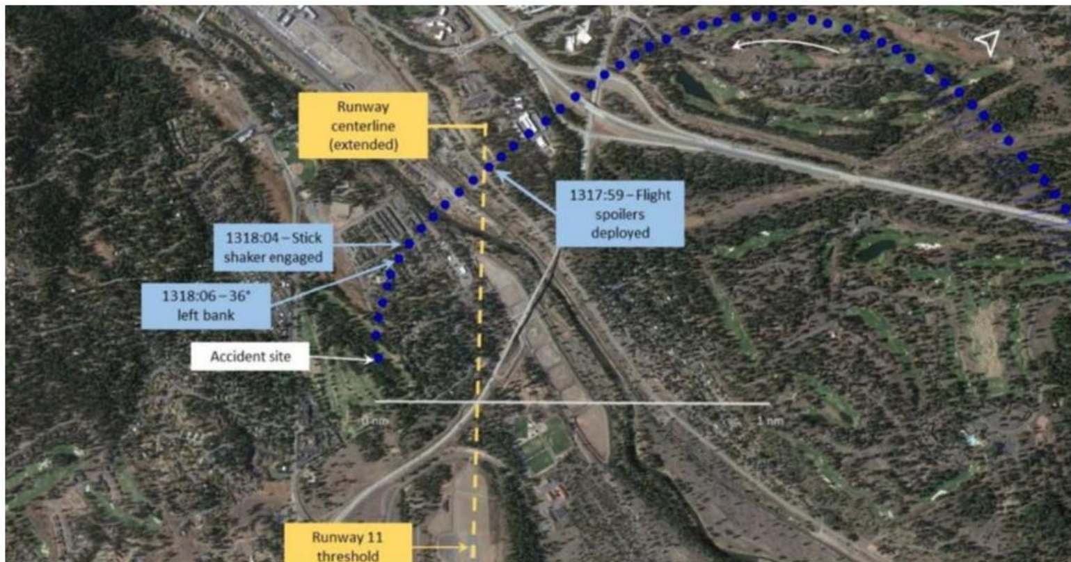
Accident airplane's flight path during final approach after crossing the runway centerline © NTSB
