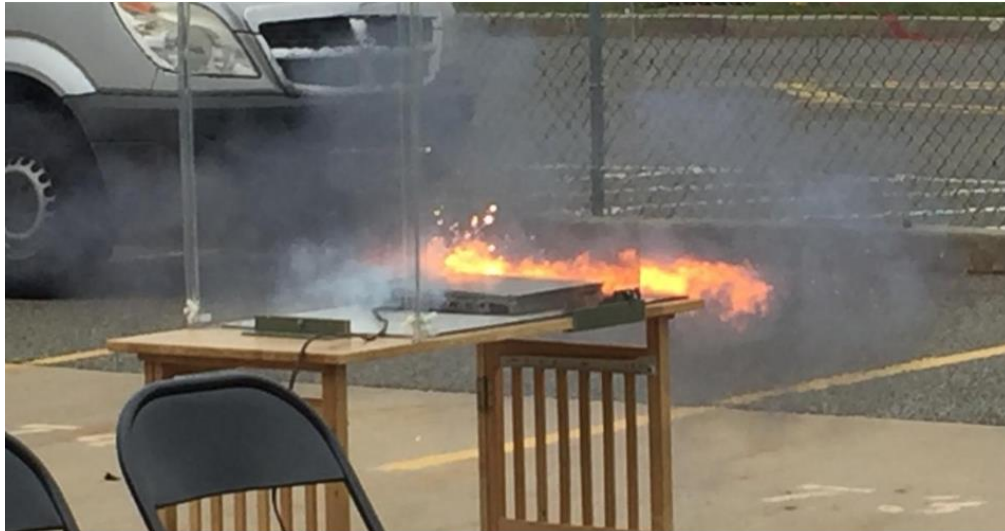
A demonstration of thermal runaway in a laptop computer under controlled conditions shows the threat these ubiquitous devices can pose to aircraft. According to the FAA, they require vigilance and an understanding of how to extinguish their fires compared to normal burns. © Curt Epstein/AIN
