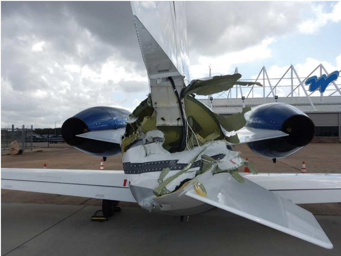
Aft view of tail cone damage to the Cessna Citation cited in the accident at Hobby Airport. Photo courtesy of NTSB.
