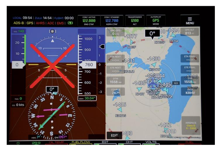
And should it happen — should the infamous red "Xs" appear, or a screen go dark — unplug and navigate to the nearest port in the storm, be that below the weather, above the weather, or on the ground at the nearest airport or airstrip. Time is not on your side. But if you are prepared, there will be time enough.
