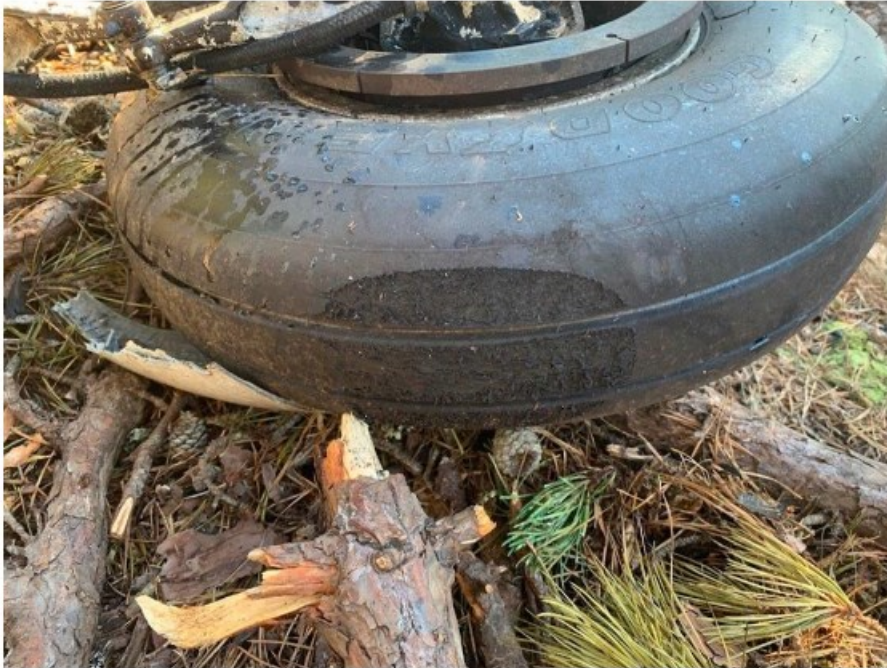
The right main landing gear tire showed areas of melted rubber.
