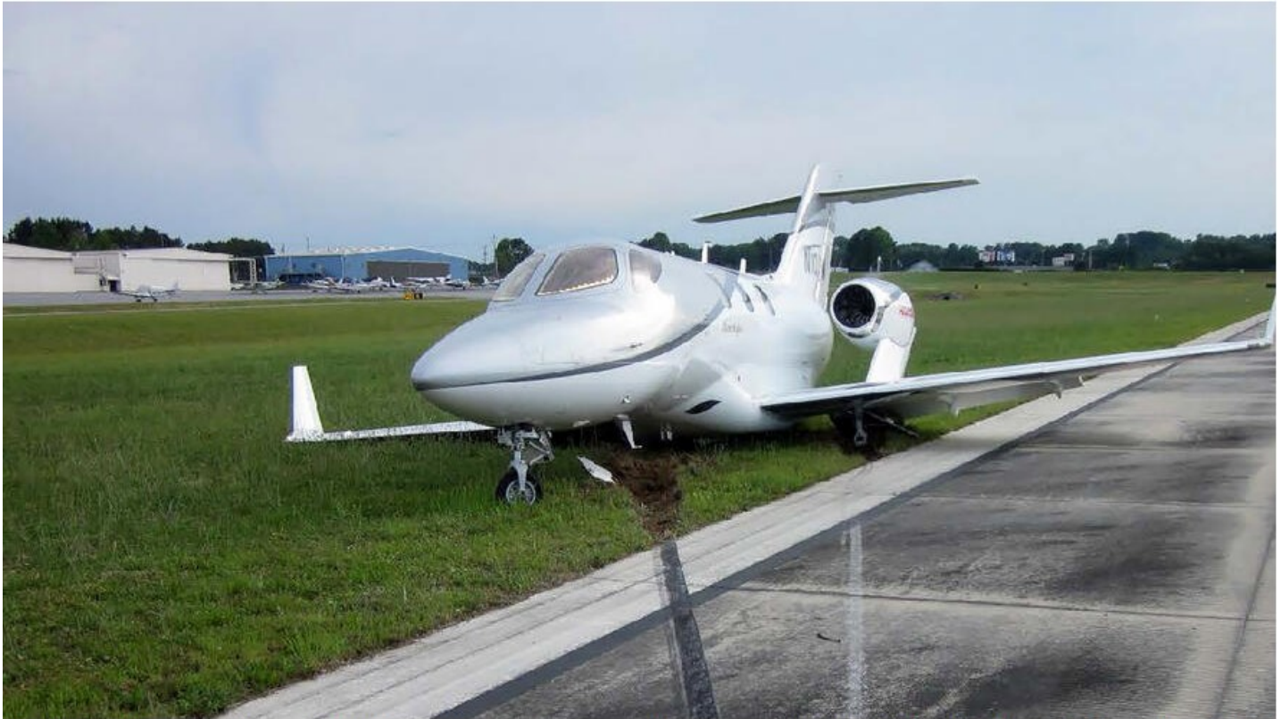
The NTSB found an improperly installed wheel caused this HondaJet to depart the runway after landing at Atlanta's Cobb County Airport. (Photo: NTSB)
