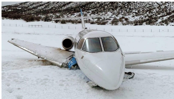
High tailwinds were a factor in this Hawker overrun at Aspen, Colorado. (Photo: NTSB)
