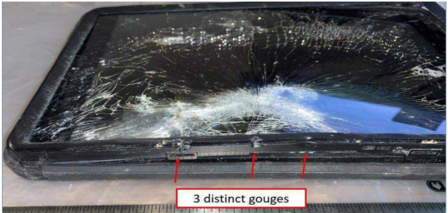
Figure 1. Condition of iPad after the accident with 3 distinct gouges in the iPad and it's case. The gouges are on the left side of the iPad when viewed in portrait mode. In the image, the iPad is rotated left into landscape mode.
