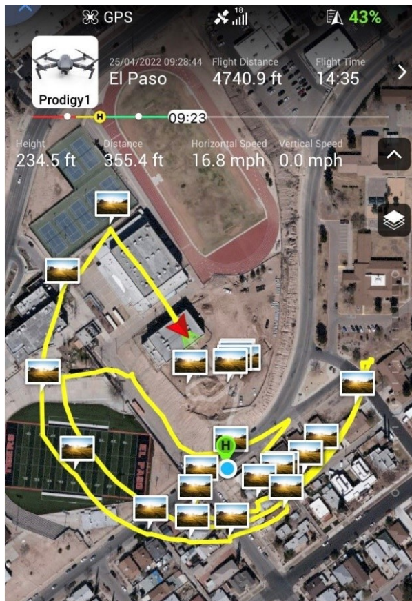
Figure 3. This is the flight path flown during the inspection of the tennis courts. The flight path illustrates how the remote pilot flew several wide arcs to the south and west of the tennis courts. (Photo courtesy of Michael McGee)
