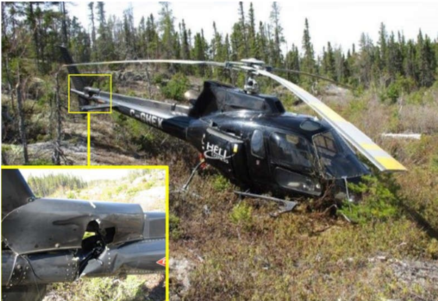
Photo of the wreckage, with inset image showing a magnified view of the damage to the tail (Photo: TSB, Sûreté du Québec)
