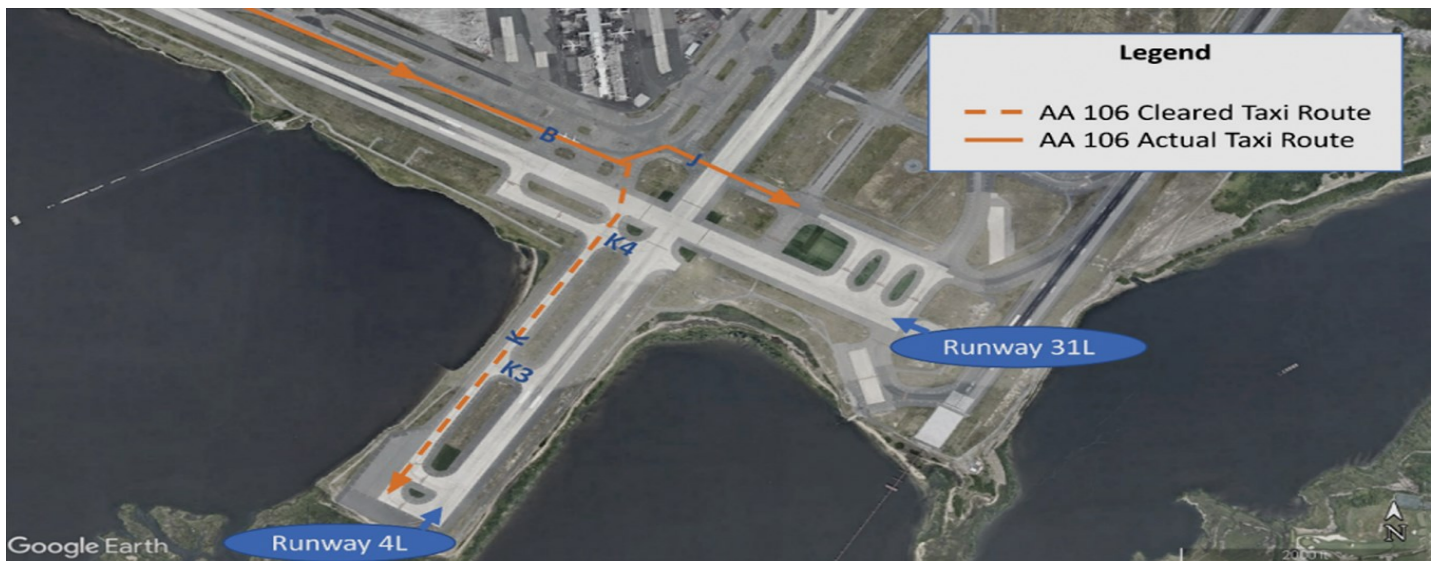
Depiction of American Airlines Boeing 777 cleared route versus the actual taxi route. Source :NTSB
